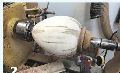
The hollowed urn is remounted for final turning after drying. Since the urn was made from green (wet) wood and the author was working on a short schedule, he sped up the drying process by "cooking" the work in a microwave oven for short intervals.
