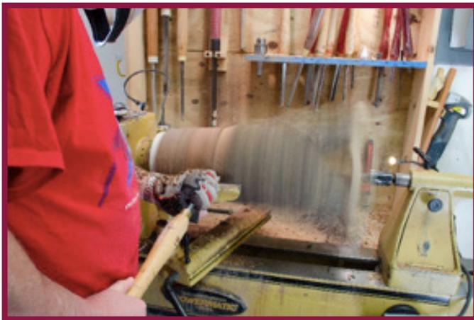
7. After the base, middle and under side of the wings are rounded and shaped, the neck and wings are turned to size. **Push Cut..**
