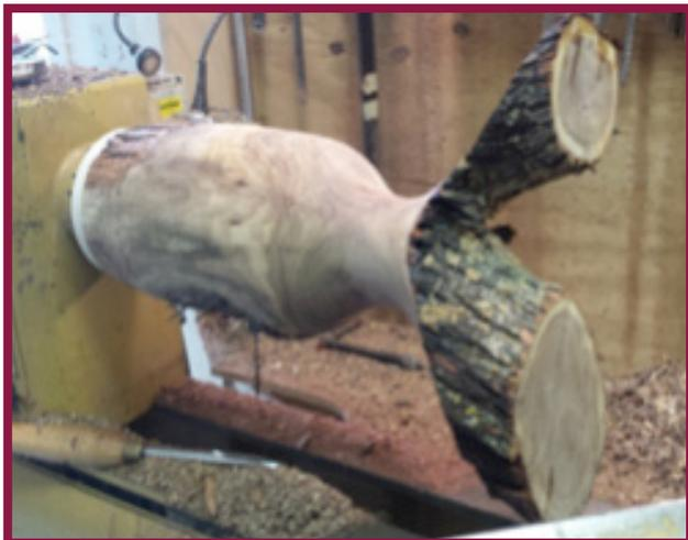
9. Steady rest is mounted and start shaping the top side of the wings of the crotch.
