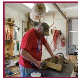
3. Mount the Crotch to the lathe with a spur center and live center on the tail stock. Aligning the crotch on the lathe so the wings and body of the vase line up evenly. bring out the best characteristics of the wood. This will maintain integrity of the shape of the vase.
