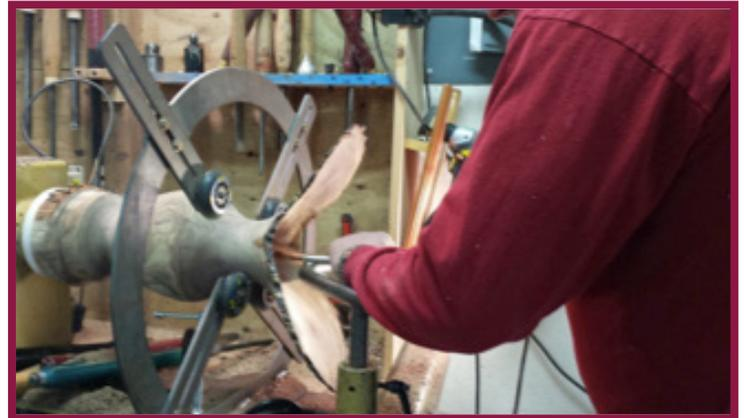
21. Turning the tendon on the base for holding onto it for final sanding.
