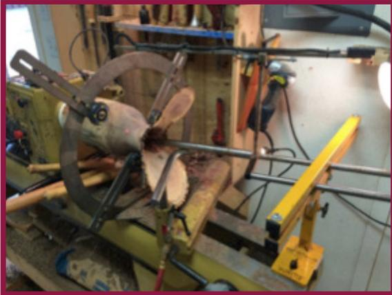
16. Remove steady rest and insert a jam chuck to support the wings of the vase while finishing shaping the bottom half of the vase.
