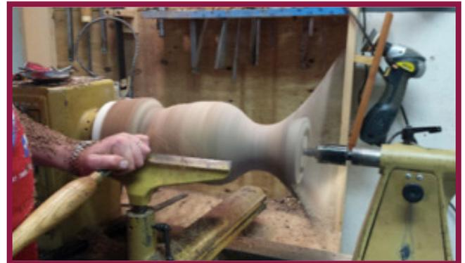
18. Put the steady rest back in place and set up the Hollowing system again to hollow out the bottom half of the vase. You can see the laser on this picture.
