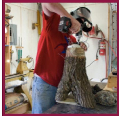
6. Rounding up the middle of the vase and shaping the underside of the wings of the crotch..
