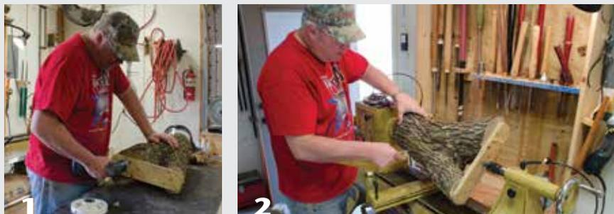
A wooden wing-support piece screwed to the top end of the branches receives the tailstock live center and allows for intentional positioning of the turning axis.
