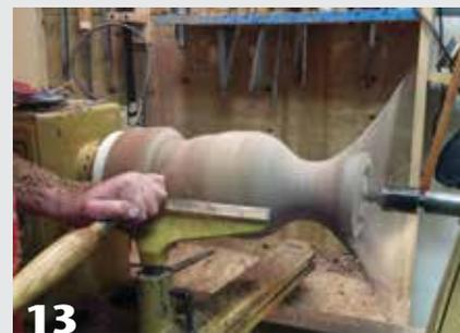
With a custom-turned, cone-shaped plug fit into the vase's opening and tailstock support in place, finish shaping the lower section of the vase's body.
