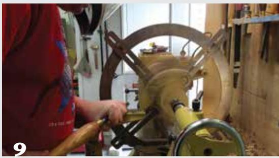
**9** View from the tailstock end shows the intermittent cutting action—air and wood.
