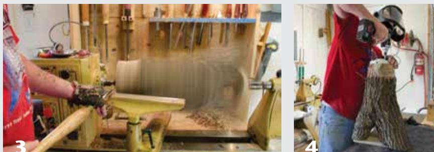
The piece is initially driven by a spur drive, allowing for adjustable positioning. Turn a flat base to accept a faceplate, the preferred and safer holding method for hollowing.
