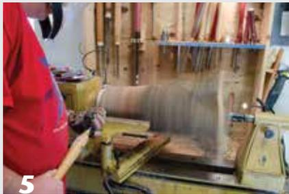
**5** With the piece mounted on a faceplate, begin shaping the lower section of the vase.
