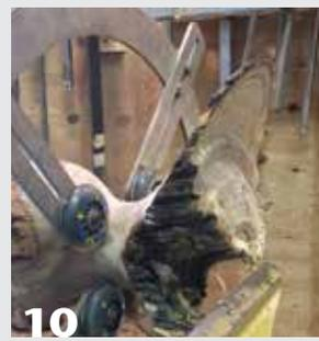
**10** Form the wings' wall thickness in stages.
